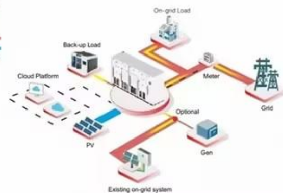
Backup side AC 4 parallel connections 130kW/261kWh*4 system
